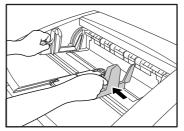
• To reset the guides so that they are equidistant from the center, spread the guides all the way to the left and right.
