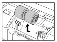
**5.** Use a moistened, well wrung-out cloth to wipe off any dirt from the roller.
