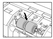
**2.** Align the notches in the roller with the shaft pins in the scanner, then slide the roller lock lever in the direction indicated by the arrow.
