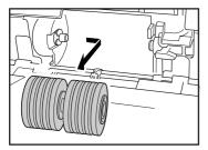
**6.** Use a moistened, well wrung-out cloth to wipe off any dust from the rollers.
