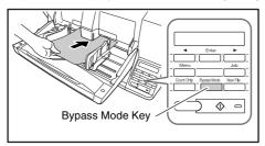
If a Feed Option other than [Standard Feeding] or [Manual Feeding] is selected, once you have started scanning, each document placed in the Document Feed Tray is scanned, and when no document is loaded, the scanner enters the standby state.
