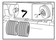
**3.** Push the feed roller lock lever up (①) and move it to the left (②) to lock the feed roller in place.
