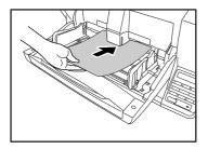
The cleaning sheet feeds through the scanner, and the Cleaning Mode exits.
