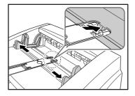
• When closing the imprinter cover, make sure that it is locked so that will not open unexpectedly. An error message appears on the display panel if the imprinter cover is open.
