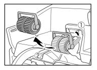
**4.** Pull the feed roller lock lever down (①) and move it to the right (②) to unlock the feed roller.
