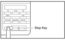
Each time you press the Stop key, the upper and lower platen rollers rotate in the following order: black  $\rightarrow$  white  $\rightarrow$  brush.
