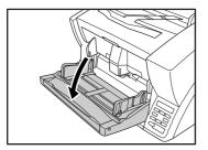
The height of the home position can be adjusted in three steps according to the number of document pages to be loaded at once (up to 500, 300, or 100 sheets). The default setting is the lowest position, which accepts up to 500 sheets. For details, refer to the *User Manual*.
