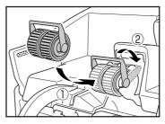
**2.** Align the notches in the shaft of the feed roller with the pins on the shaft in the scanner, and place the feed roller into position.
